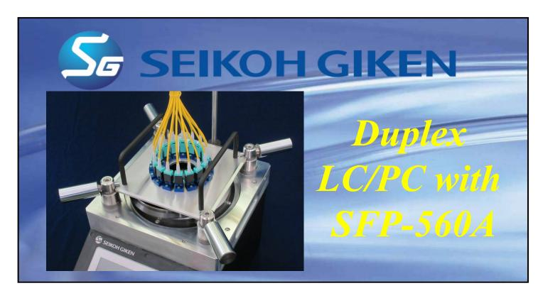
Polishing Holder: PH55-PL-32DFX (Fixed type holder with metal adapter)
